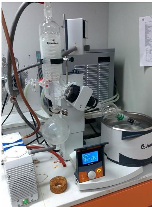
1. Power on the rotovap, the water bath, and the rotovap chiller. Generally the chillers take about 20 minutes to cool down the 50:50 water:ethylene glycol coolant.
