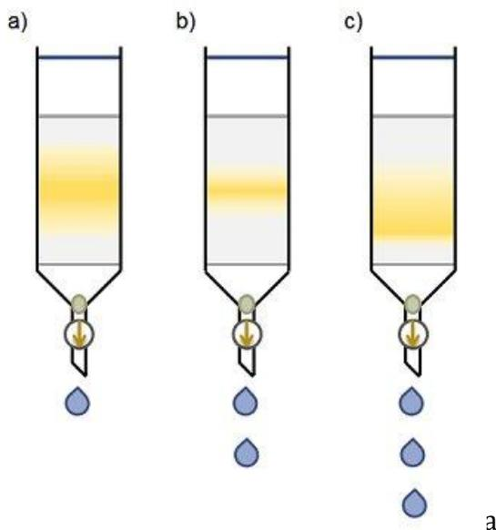
*Changing the flow rate can alter the quality of the separation. Optimal flow rate is shown in b).*
